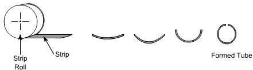
Fig 11.10: Forming of Tube from Strip
